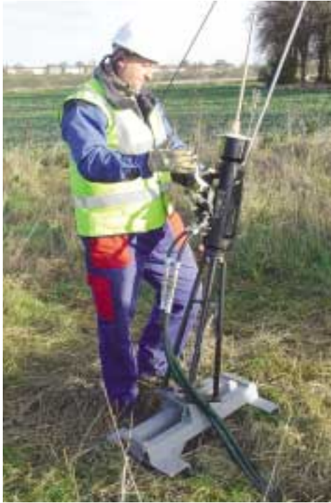
Fast and efficient loading of the anchor. No bending or squatting – all at eye level.
